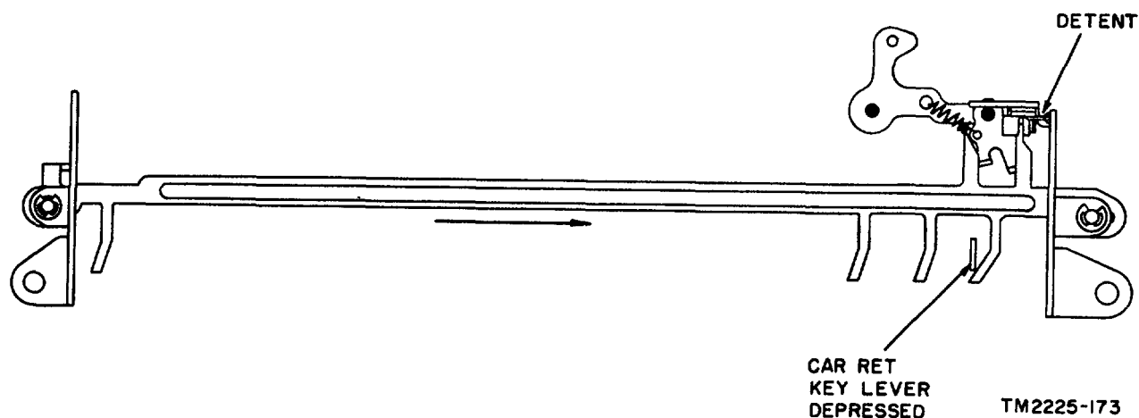
Figure 2-18. Function blocking bar, CAR. RET. key lever depressed (TT-76/GGC, TT-76A/GGC, and TT-76B/GGC serial Nos. 255 and below, Order No. 13931-PC-58).
